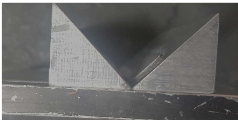
Figure 7.9: Wedge target holder used in experiments.
