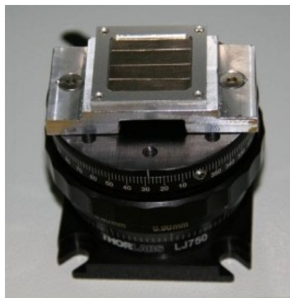
Figure 6.2: Americium source placed on a calibrated vertical translation platform.
