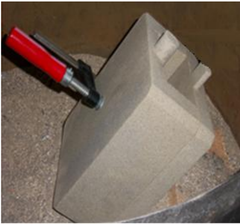
Fig. 2. Sand mould tilted 60° from horizontal.
