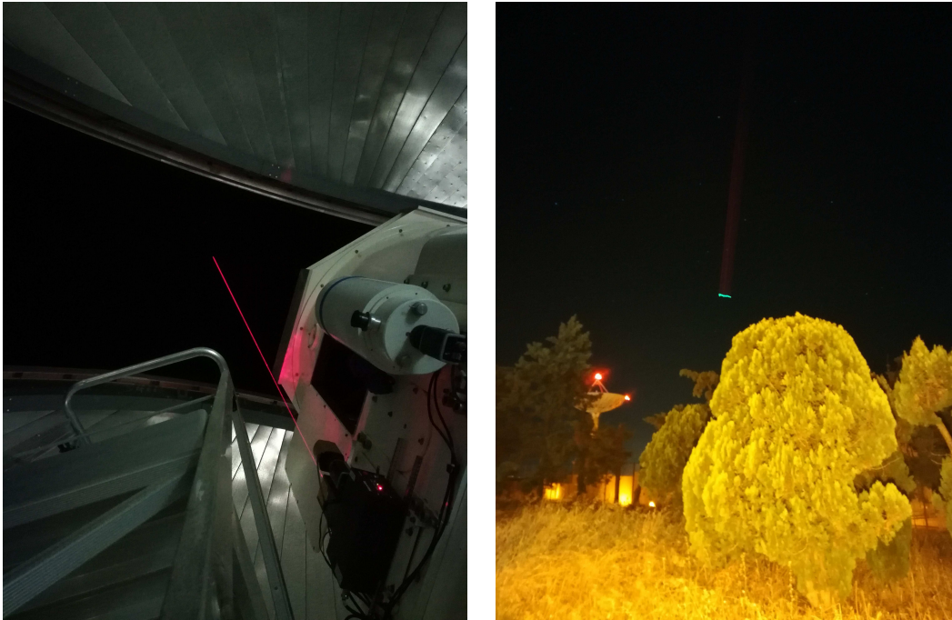
Figure 4.14: (left panel) The red beacon laser mounted on the MLRO telescope. (right panel) Micius satellite during the passage.
