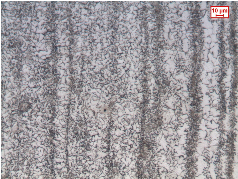
Figure 3.36. Micrograph of the interface between HAZ and base material at 200x. A dense segregation of pearlite and ferrite, due to the rapid cooling, is appreciable.
