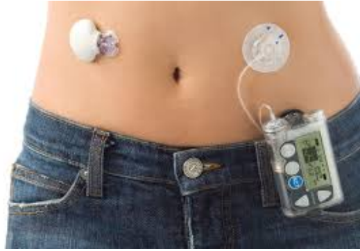
FIGURE 5.1: A commercial subcutaneous glucose sensor (CGM, on the left) and a commercial insulin pump (on the right). The pump is connected to a subcutaneous needle via a catheter.
