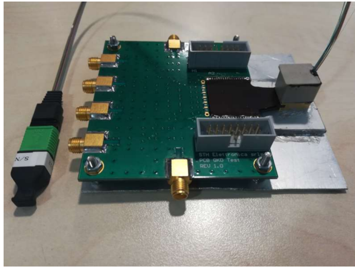
Figure 8.12: Photo of the PIC assembled on the connectorized RF PCB.
