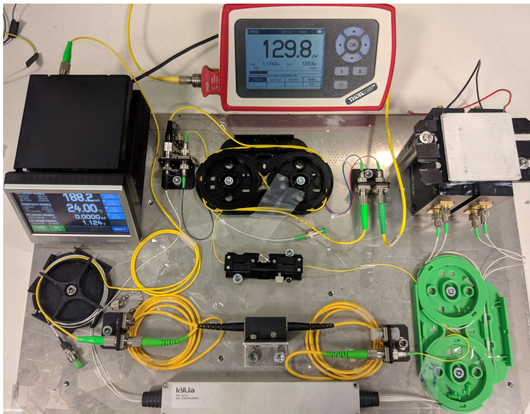
Figure 3.11: Photo of the actual setup. On the top left we can see the controller of the laser with the laser source used for the LO. In the center is possible to see, starting from the bottom, the 90 degree hybrid in its metallic enclosure, the variable optical attenuator, the polarization controller, the fiber beamsplitter and the power meter used to monitor the power of the LO. Finally, on the top right are visible the two balanced detectors.
