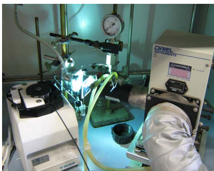
Figure 2.15. Photoreactor working in continuous with trans-membrane flow collecting.
