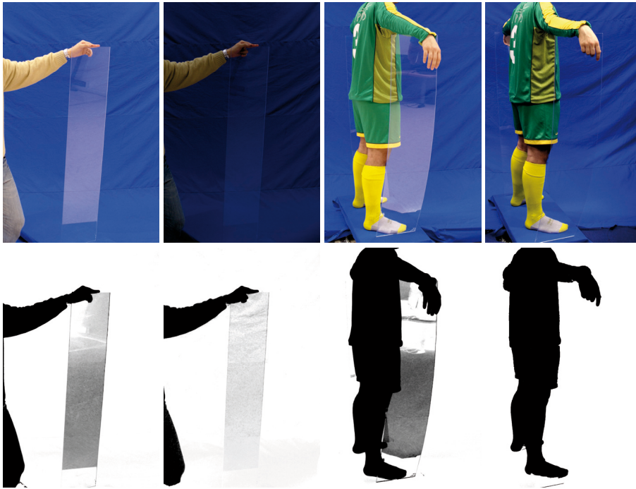
Figure 3.4: Specular reflections generated by the plexiglas plates and their influence on the colors and the segmentation results.
