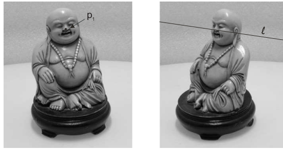
Figure A.13: Left and right images of a stereo pair: \ell is the epipolar line associated to p_1 .
