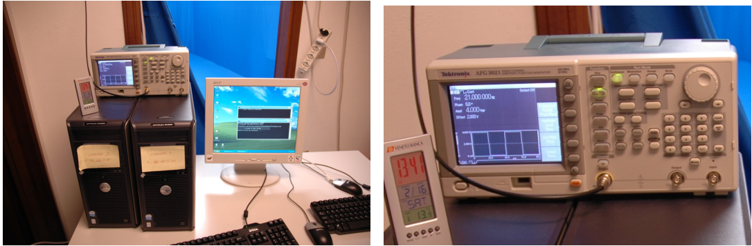
Figure 5.10: (Left) Control room setup. (Right) Digital function generator used as trigger for the synchronization system.
