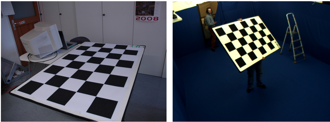
Figure 5.11: (Left) Checkerboard used in the calibration stage. (Right) A calibration photo taken at low brightness to increase the corners detection accuracy.
