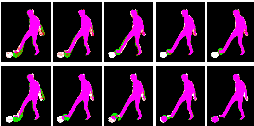
Figure 6.8: Evolution of the algorithm during an estimation of the pose represented by the white silhouette. (Top row) No shape information is used to compute the silhouettes correspondences. (Bottom row) Shape matching metric is used.
