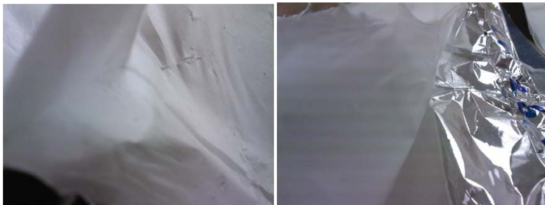
Figure 108 Peeling of the membrane from the alluminium foil (a) membrane based on electrospun PMMAcoMAA; (b) membrane based on electrospun PANcoVAc
