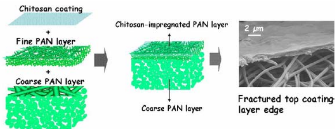
Figure 35 Fabrication schematics of the electrospun PAN scaffold with a chitosan coating layer.
