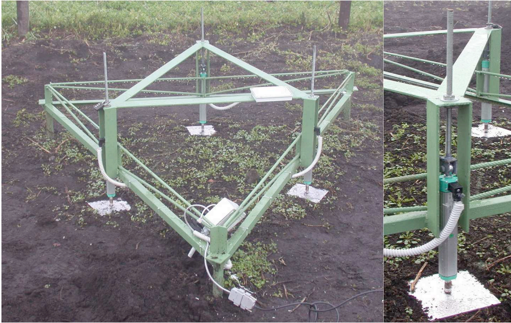
Figure 3.1: Steel tripod constructed to continuously monitor the elevation changes of the peat surface. A zoom of the displacement transducer is shown on the right. The anchoring piles and the displacement transducers are highlighted.
