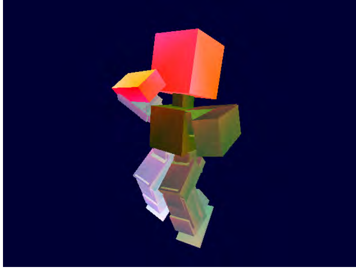
Figure 5.7: Output of the collision prevention system. The figure shows the motion that would be generated if the collision prevention system were not enabled and highlights the colliding parts by a red color.
