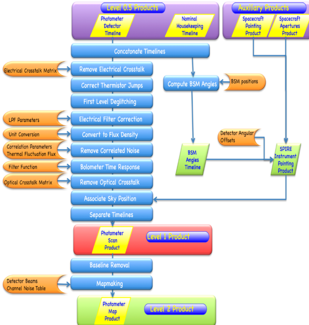
Figure 3.11: Flowchart for the Large Map, Small Map and Parallel mode data processing pipelines. Data products delivered to the user are shown in yellow, intermediate data products in green. Processing steps are shown as light-blue boxes while calibration files are shown in orange (Spire Observers’ Manual 2010).
