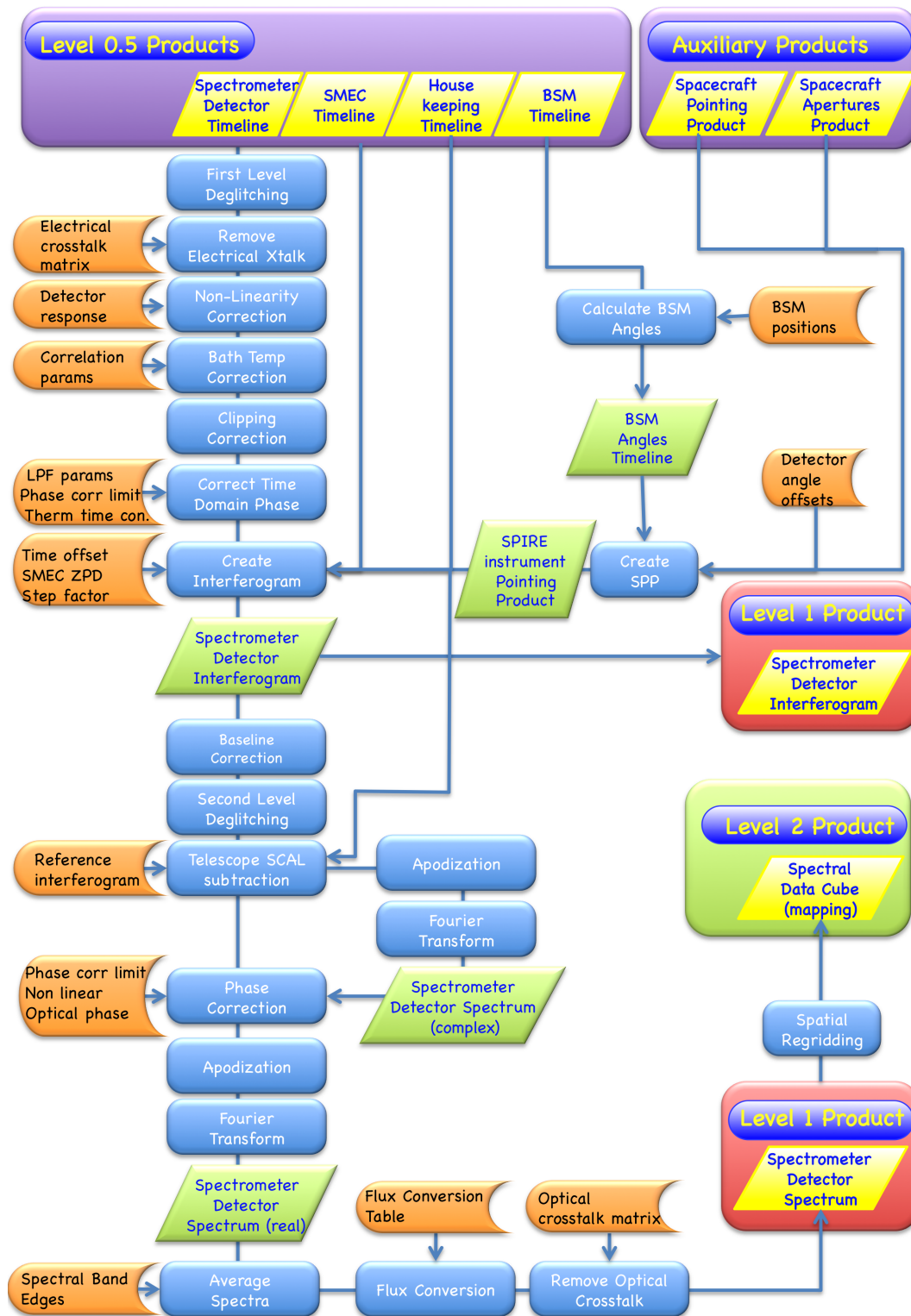
Figure 3.18: SPIRE Spectrometer pipeline flow. Data products delivered to the user are shown in yellow, intermediate data products in green. Processing steps are shown as light-blue boxes while calibration files are shown in orange (Spire Observers' Manual 2010).
