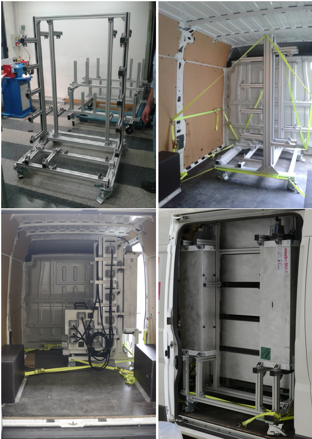
Figure 5.18: Different stages of MODES-SNM mounting on the chassis and inside the van: the chassis made by Uninsubria (upper left panel), testing the final position (upper right), with the system mounted view from the rear (lower left) and view from the side door (lower right)
