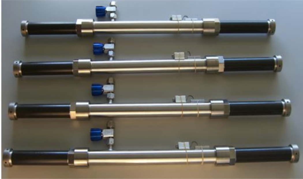
Figure 2.22: ^4\text{He} fast neutron tubes used in MODES_SNM
