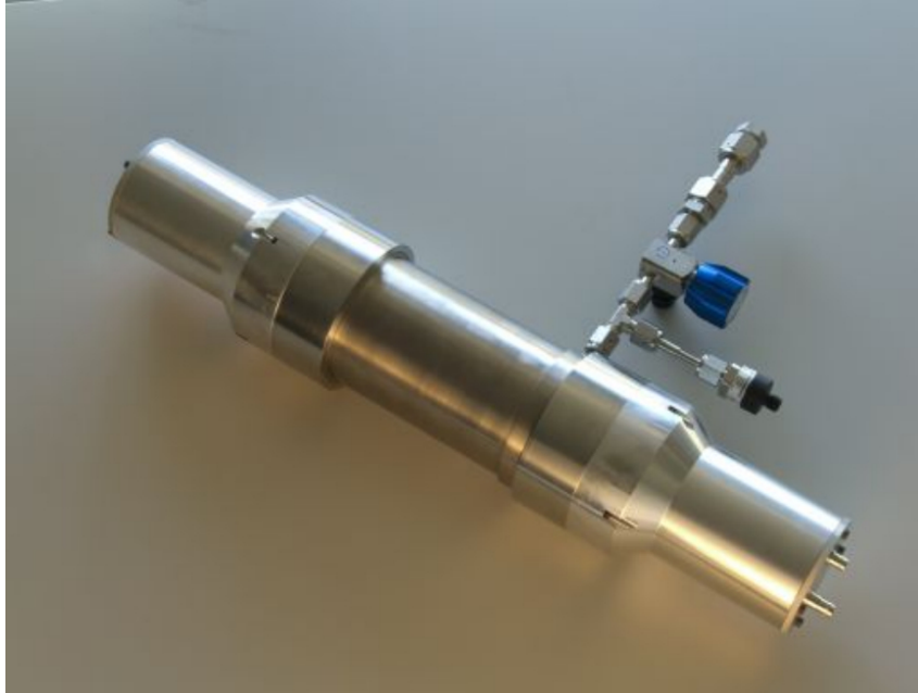
Figure 2.5: The xenon gamma-ray detector used in MODES_SNM
