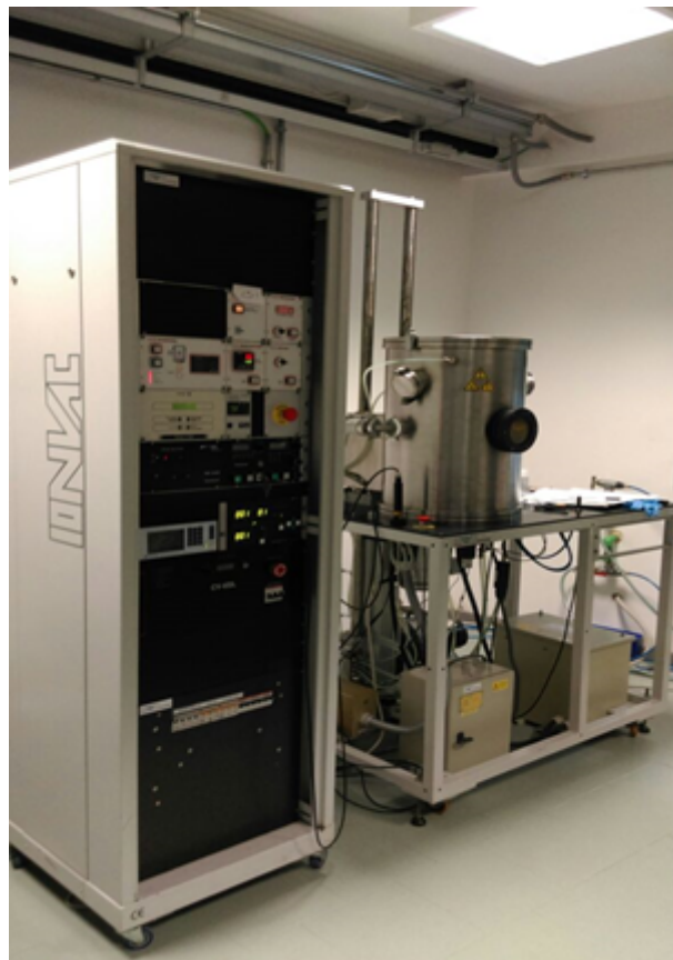
Figure 3.5: E-beam chamber system at LUXOR laboratory.
