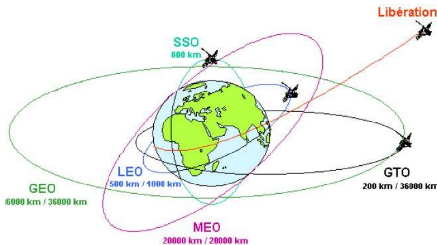
Figure 36: Different possible orbits of satellites, including the LEO in blue.
