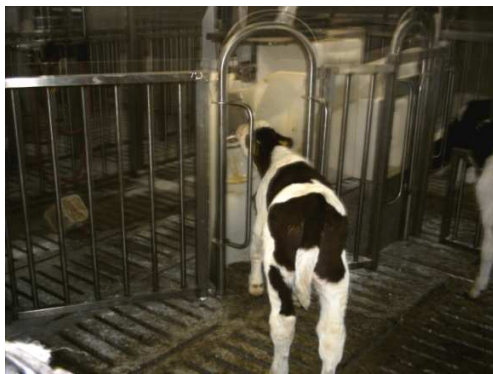
Figure 1.9 Automatic milk feeding device for veal calves.
