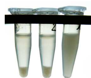
Fig. 4.25 HA precipitation from pT7, pT7hasA-tuaD and pT7hasA-tuaD-gtaB-pgi transformed E.coli culture medium by absolute ethanol. pT7 E.coli (eppendorf 1) no produce HA (control).
