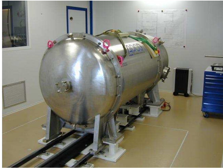
Figure 2.3: HARPS, the High Accuracy Radial velocity Planet Searcher, is a fibre-fed high resolution echelle spectrograph for the measurement of radial velocities with the highest accuracy currently available.
