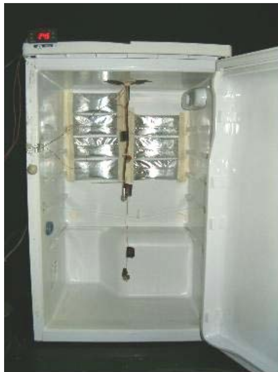
Figure 3.1.3 The prototype with 70% of the total PCM. Two configurations
