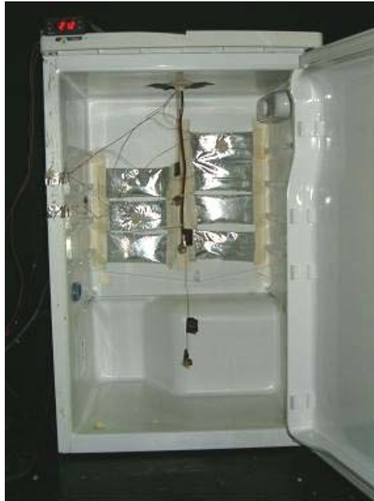
Figure 3.1.4 The prototype with 70% of the total PCM. Two configurations
