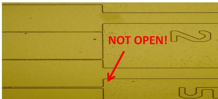
Figure 5.9: Test structure with incomplete development after exposure and post-exposure bake. The 5\mu\text{m} channel looks open but actually it is not.
