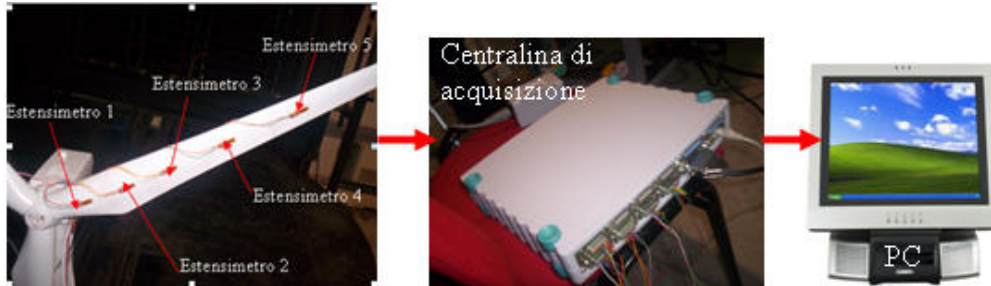
Figure A6: Strain gauge measurement chain.
