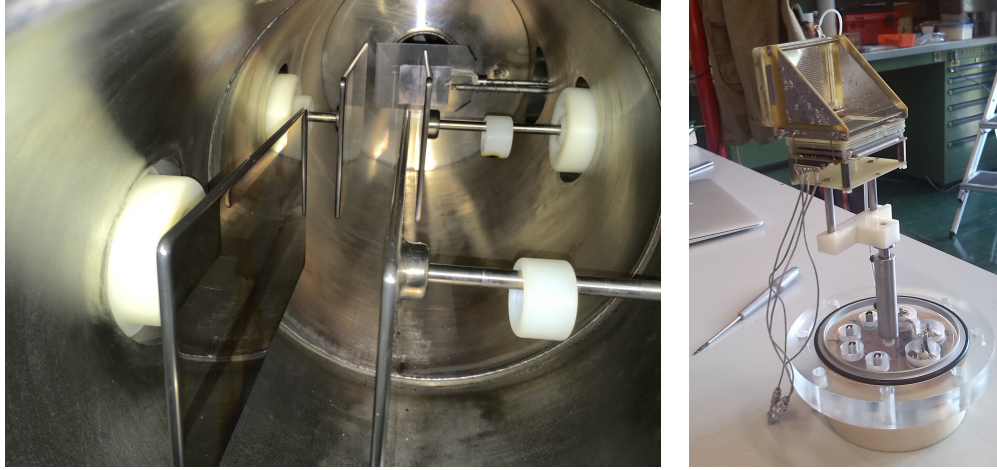
FIGURE 4.4: The internal part of the electrostatic deflector with the two pairs of electrodes (left) and a picture of the MCP in use (right).
