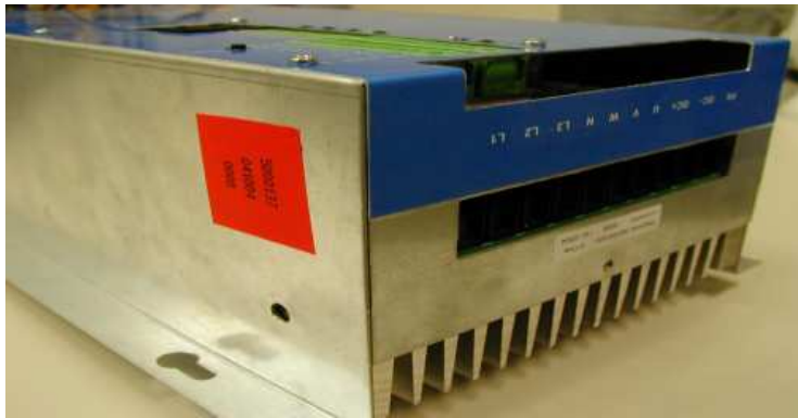
Figure 3.5: Inverter prototype use to create the lift equipment
