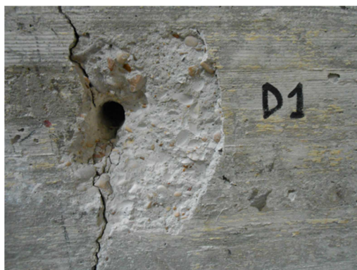
Figure 3.38 Failure mode of AC2 specimen after test session 1. Load vs displacement graph for AC2
