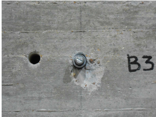
Figure 3.18 View of MEC5 specimen after test session 3. Load vs displacement graph for MEC5
