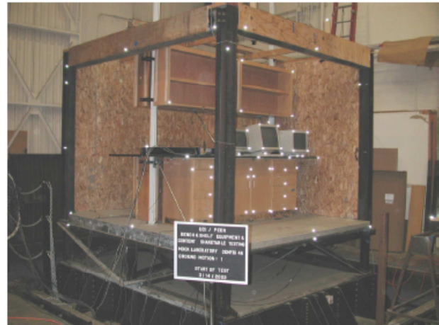
Figure 1.58 Dynamic testing on office equipment (Comerio 2005)
