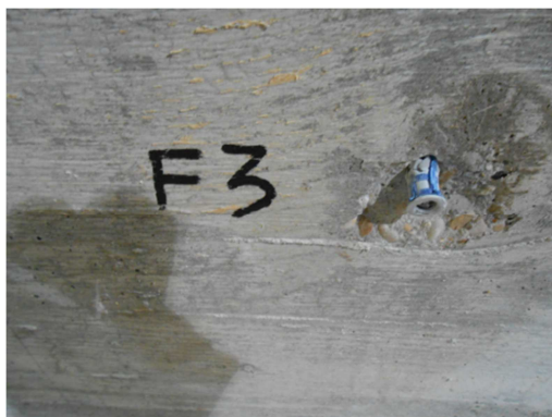
Figure 3.62 Failure mode of PFEC1 specimen after test session 3. Load vs displacement graph for PFEC1
