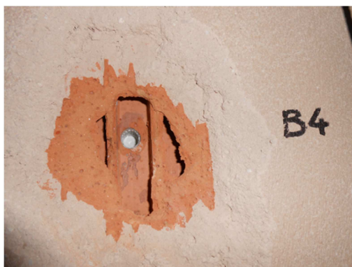
Figure 4.10 Failure mode of AM2 specimen after test session 4. Load vs displacement graph for AM2
