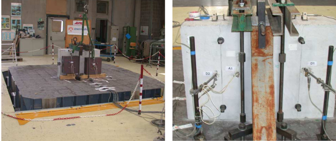
Figure 1.40 Shake table testing of three anchor types (Rieder 2009)
