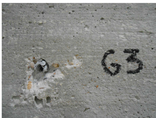
Figure 3.54 Failure mode of PEC5 specimen after test session 3. Load vs displacement graph for PEC5
