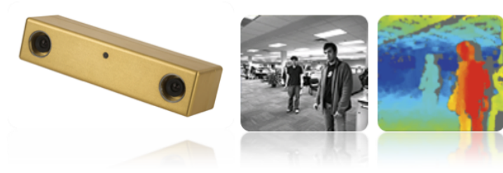
FIGURE 2.3: Bumblebee stereo camera. The depth of observed surfaces is triangulated from the slight visual differences in the two camera frames. The depth image quality of passive stereo cameras is inferior with respect to cameras that exploit active structured light projection but unlike these can work outdoor without issues.
