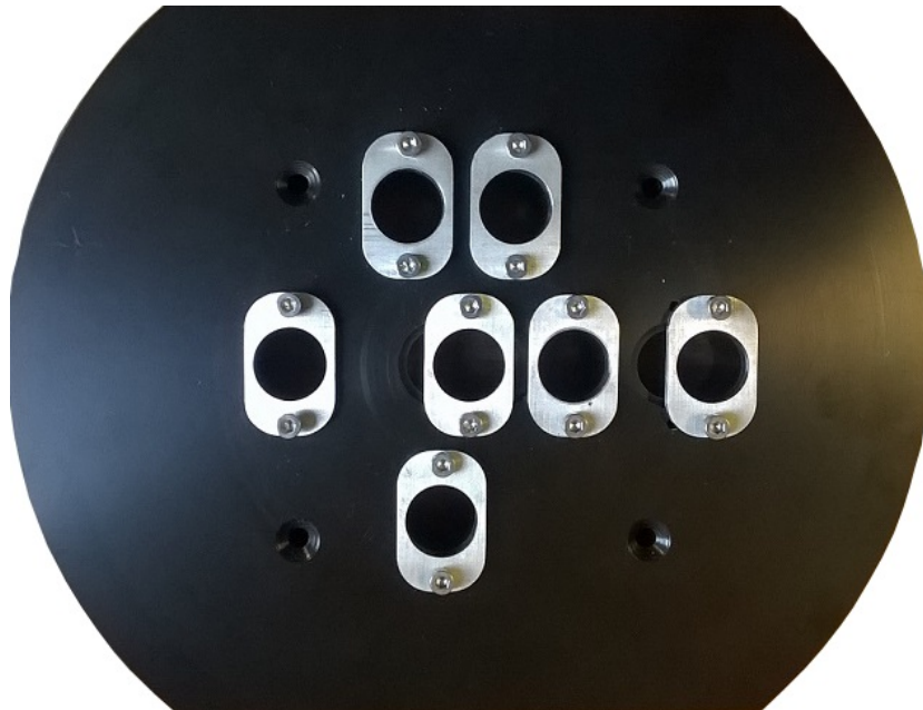
Figure 4.8: Prototype of the support for the optic heads dedicated to the OES diagnostic in SPIDER.
