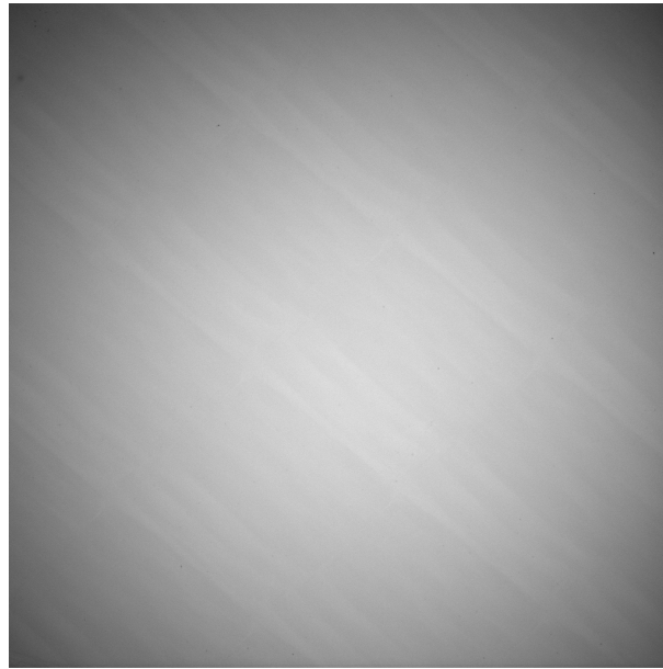
Figure 4.1: Example of acquisition of a uniform illumination field, t_{exp} = 0 ms, t_{open} = t_{close} = 50 ms.
