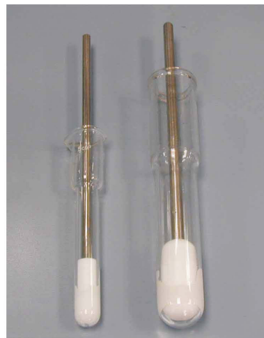
Figure 1 | Glass/Teflon Potter Elvehjem homogenizers. The homogenizer on the left (5 ml) is most suitable for isolation of mitochondria from cells, whereas the one on the right (30 ml) is more appropriate for isolation from tissues.
