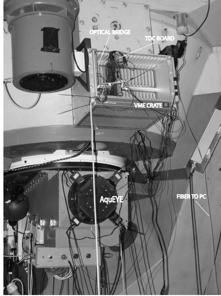
Figure 7.5: AquEYE mounted at the Asiago telescope. On the top the electronics with the TDC board and the optical bridge, on the bottom the instrument with the four SPADs.
