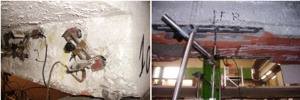
Fig. 4.2: Example of strain transducers applied to the embedded truss (a) and of inductive displacement transducers applied to the under the beam mid-span section (b)
