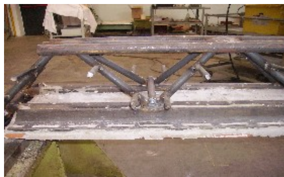
Fig. 4.31: particular view of a nude truss beam head
