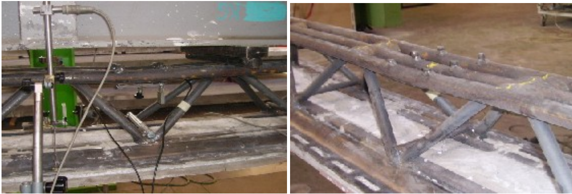
Fig. 4.35: Pictures of the local buckling happened in the second truss 102n
