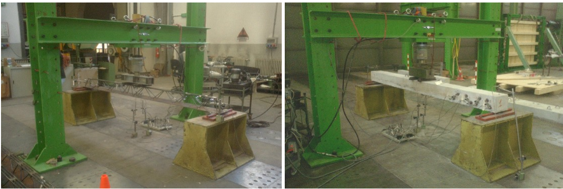
Fig. 4.6: Pictures of a REP ® -NOR truss (a) and a REP ® -NOR composite beam (b)
