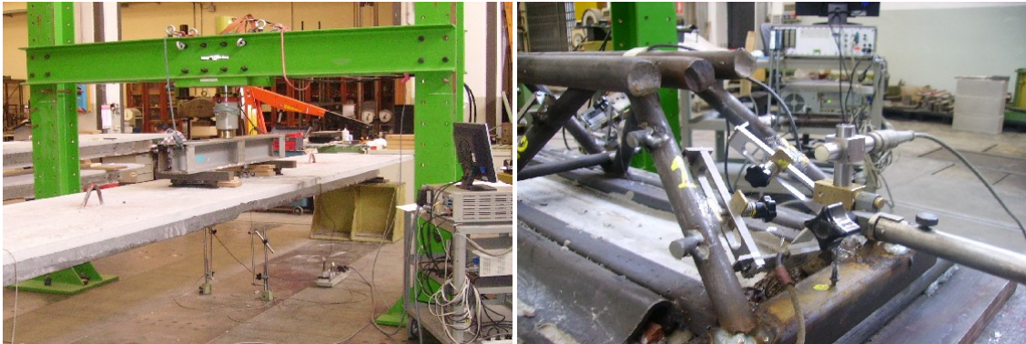
Fig. 4.1: Load frame with hydraulic jack, load cell and distributor beam (a) and example of strain transducers applied to the nude truss (b)
