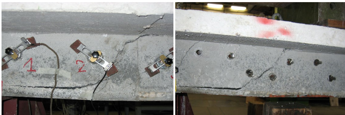
Fig. 4.52: Pictures of the composite beam 103 after their collapse
