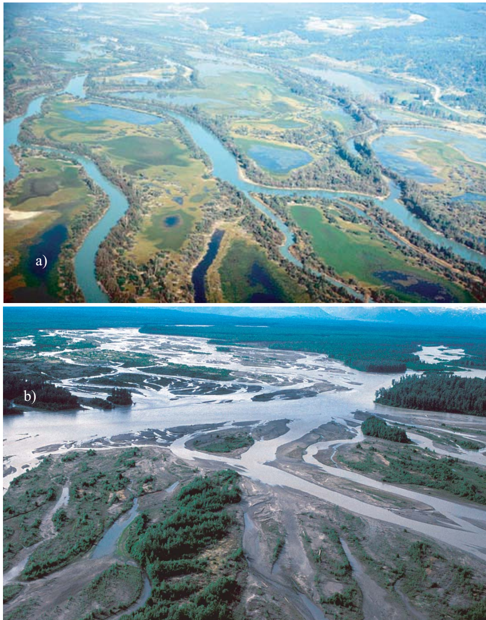
Figure 1.11: Typical examples of anastomosing rivers: a) Columbia River, British Columbia, Canada; b) Matanuska River, Alaska, USA.
