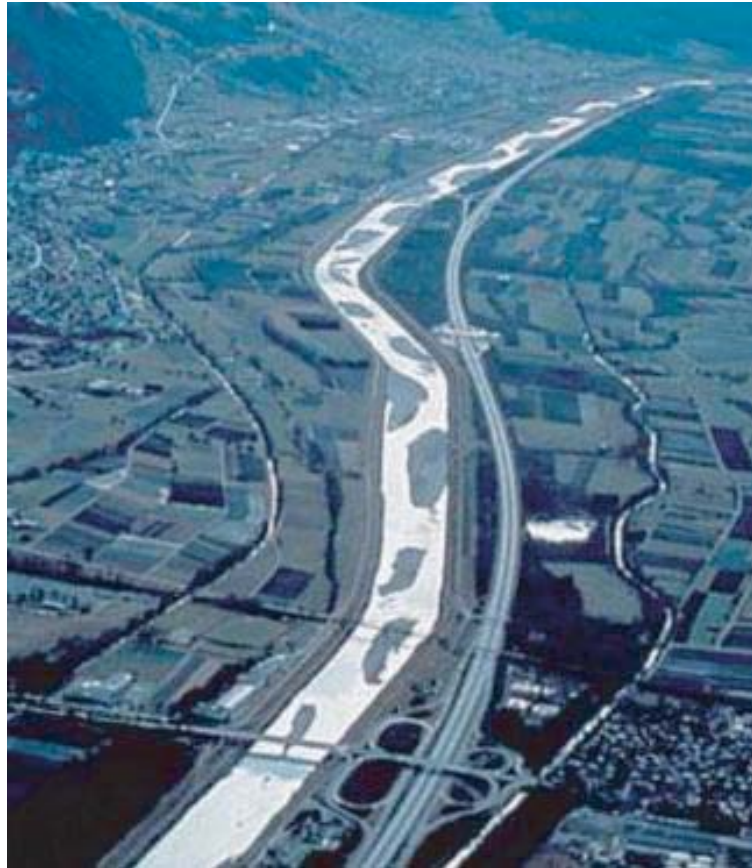
Figure 1.2: Alternate bars in the Rhine River, Switzerland [Jaeggi, 1984]
