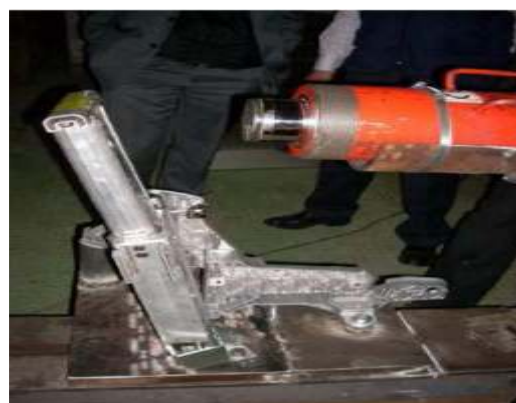
Fig. 3.48: final configuration of the testing assembly after the test.
