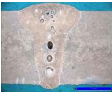
Fig. 5.14: EBW seam. Test 3, single run. Castasil®-37.
