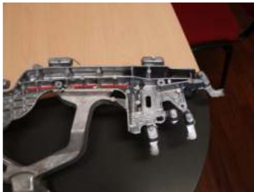
Fig. 3.95: connection ingate/casting with modified radii.
