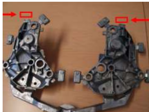
Fig. 3.80: enlarged overflows on the two cavities. Moving die.
