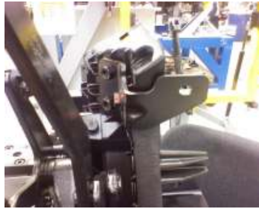
Fig. 3.46: the fixing of the carrier on the roll bar of a F149 RTH.
