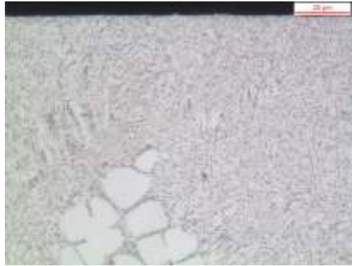
Fig. 4.49: externally solidified dendrite. Plate C1. 500X.
