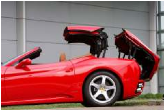
Fig. 3.1: the 5-part RTH of the Ferrari F149.
