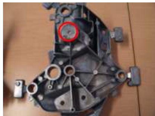
Fig. 3.77: elimination of the hole. Sight of the moving die.
