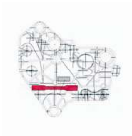
Fig. 3.10: positioning of the tensile specimen of the roof main bracket.
