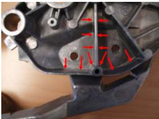
Fig. 3.79: ingate area and rib. Sight on the moving side of the die.
