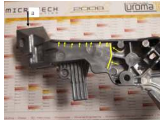
Fig. 3.103 increasing the inclination of die. Moving slide.
