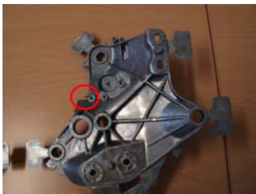
Fig. 3.76: the re-introduced steel core Fix die.
