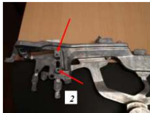
Fig. 3.92: elimination of steel cores. Fix side frame die.
