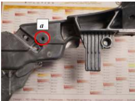
Fig. 3.100: broken pin. RH Side frame.
