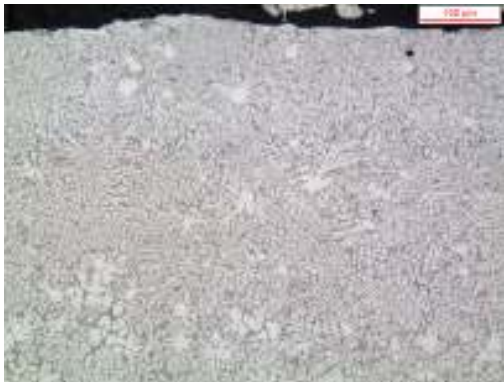
Fig. 4.50X: HSTRC microstructure. Edge. 100X.
