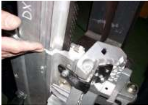
Fig. 3.49: the bearing bush before the test.
