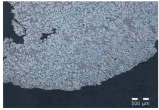
Fig. 3.28: section B; the metal has been visibly compressed. HF 1 %.
