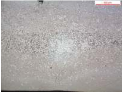
Fig. 4.43: segregation of eutectic. 25X.
