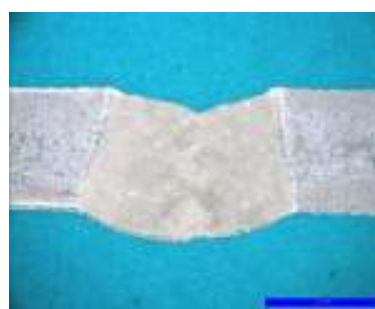
Fig. 5.6: LBW seam. Test 4. Castasil ® -37.
