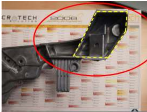
Fig. 3.102: increasing the inclination of die. Side frame.
