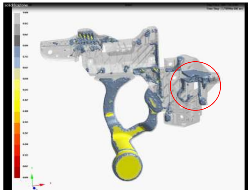
Fig. 3.113: fraction solid in position A, according to a CAD simulation.
