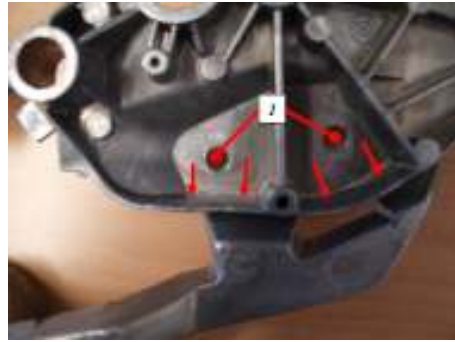
Fig. 3.78: the polished area in the ingate and the points where flashes have been introduced. Sight on the moving die.
