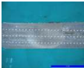
Fig. 5.22: micro-hardness profiles on a 4 mm thick plate.
