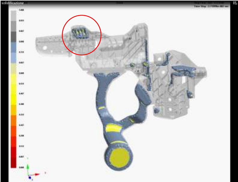
Fig. 3.115: fraction solid in position B according to the simulation.
