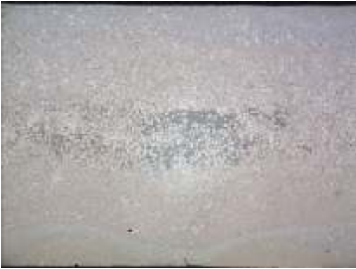
Fig. 4.44: segregation of eutectic. 25X.
