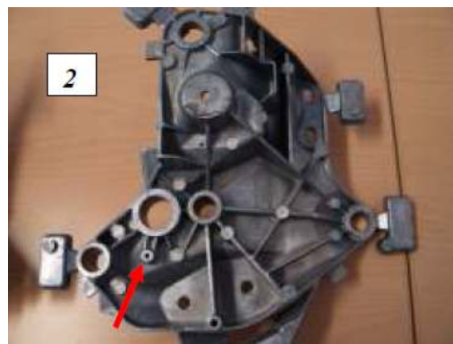
Fig. 3.72: removed steel core of the roof main bracket. Sight of the moving die.
