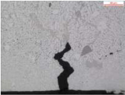
Fig. 4.48: crack initiation at the border of plate C1. Zoom of fig. 4.47. 200X.
