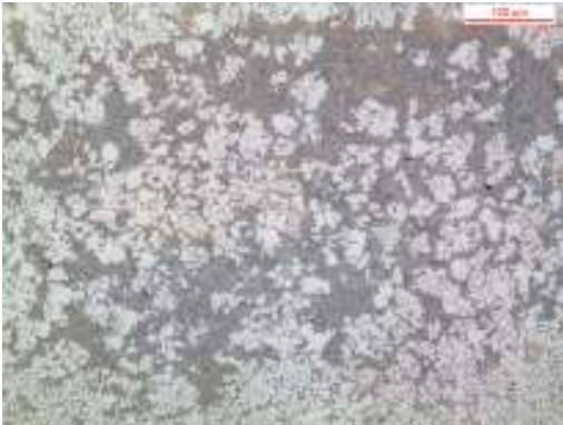
Fig. 4.46: segregation of eutectic. 100X.
