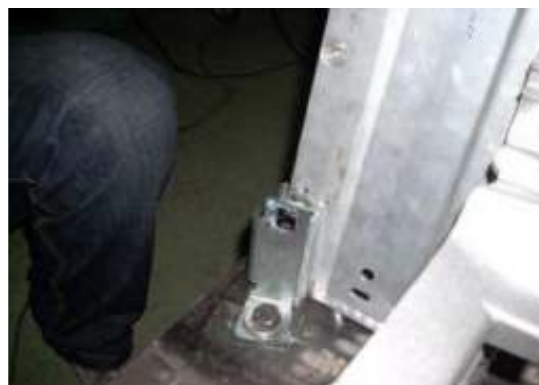
Fig. 3.53: broken fixing point roll bar to test bench.
