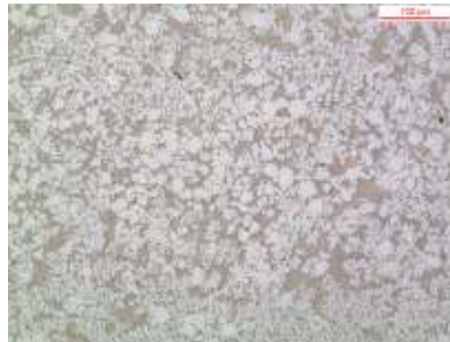
Fig. 4.51: HSTRC microstructure. Core. 100X.
