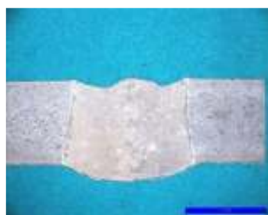
Fig. 5.5: LBW seam. Test 2. Castasil ® -37.
