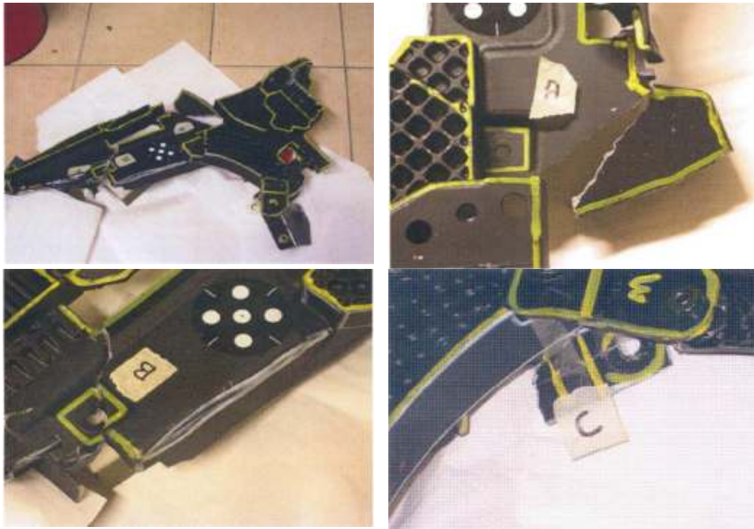
Fig. 3.24: the carrier 1 with its three fractures (up-left). Fracture A on the lower anchoring point to the roll-bar (up-right), fracture B in the area where tensile bars are cut-off (low-left), fracture C on the upper anchoring point to the roll-bar (low-right).
