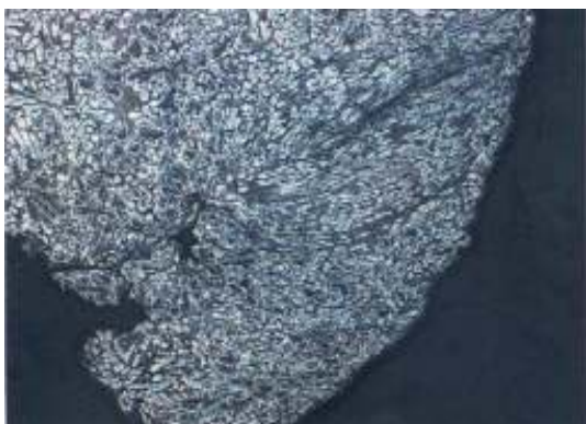
Fig. 3.29: section B; the metal has been visibly compressed. HF 1 %.
