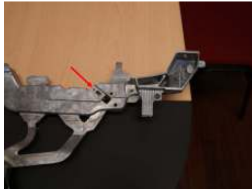
Fig. 3.94: steel core and slide position of the RH side frame.
