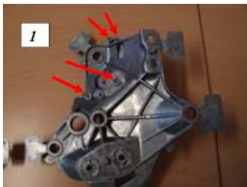
Fig. 3.71: removed steel cores of the roof main bracket. Sight of the fix die.
