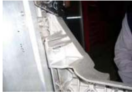
Fig. 3.50: the connection carrier-roll bar after the test. Heavy deformation is visible.
