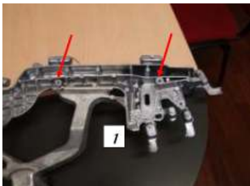
Fig. 3.91: elimination of steel cores. Moving side frame die.
