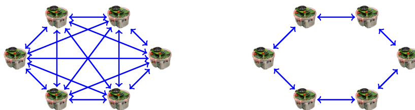
Figure 1.12: On the left, a multi-agent system where all the agents communicate with all the others. On the right, a system where an agent communicates only with the two nearest neighbors. The convergence speed of the same distributed algorithm in these two different situations can be dramatically different.
