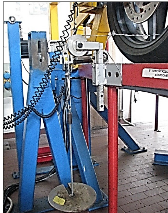
Figure 29: Lateral stiffness test
