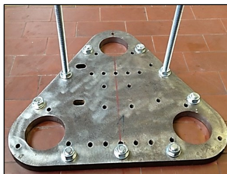
Figure 61: Base plate fixed on the ground
