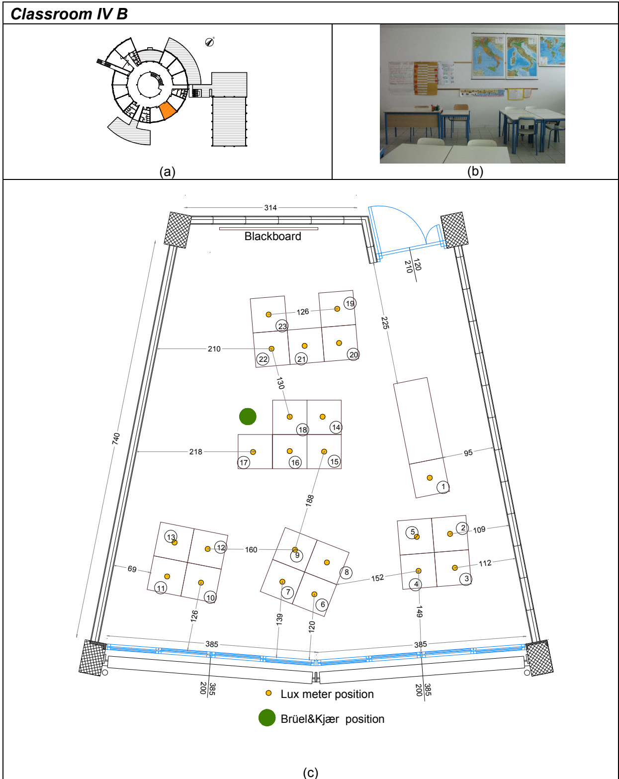
Figure 6.20 - Classroom IV B (Ceggia): key plant (a); photo (b); desks layout and position of the Indoor Climatic Analyser Bruel&Kjaer and of the Minolta luxmeter (c)
