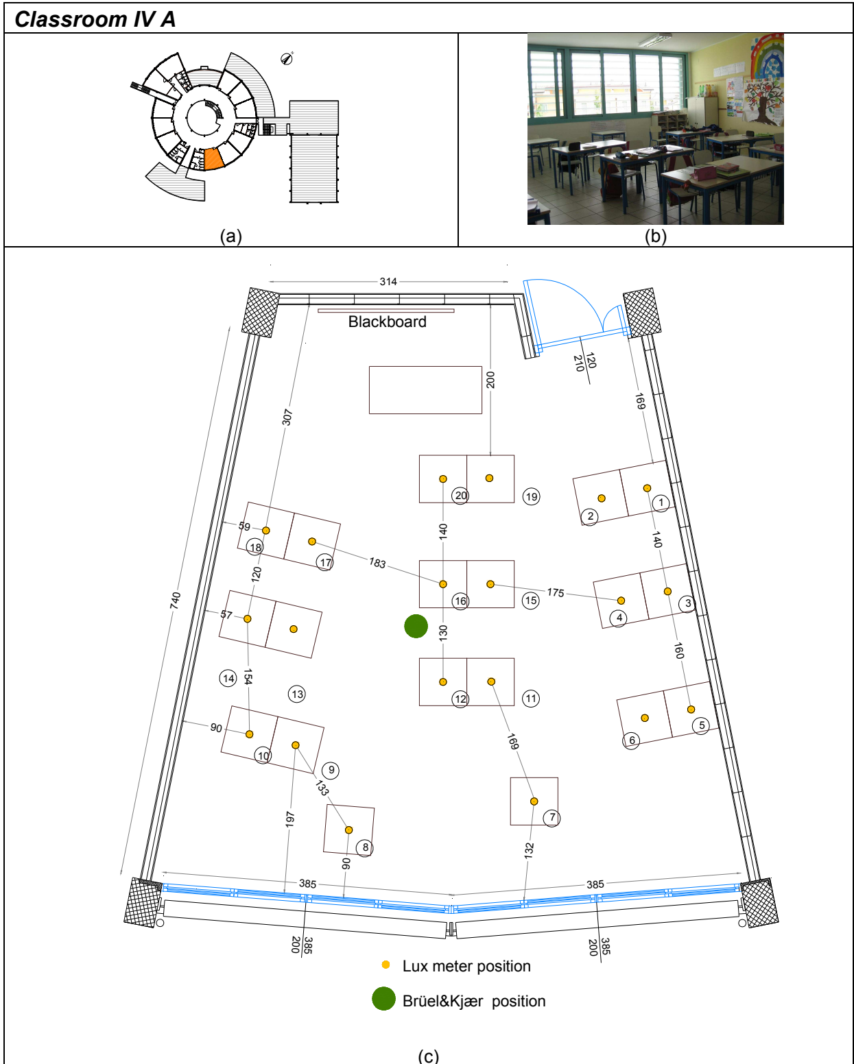
Figure 6.17 - Classroom IV A (Ceggia): key plant (a); photo (b); desks layout and position of the Indoor Climatic Analyser Brüel&Kjær and of the Minolta luxmeter (c)
