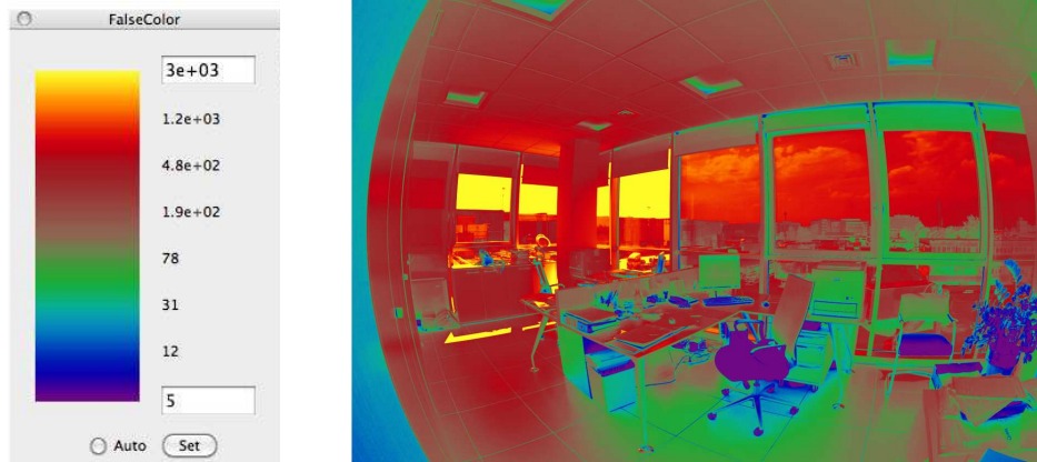
Figure 5.56 - False colour image which maps the luminance distribution of the office (a) in Figure 5.55
