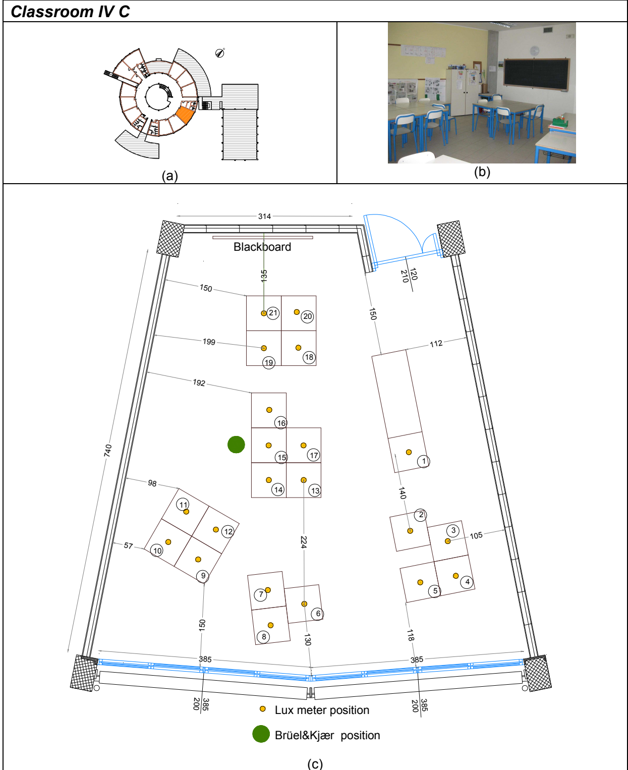
Figure 6.23 - Classroom IV C (Ceggia): key plant (a); photo (b); desks layout and position of the Indoor Climatic Analyser Bruel&Kjaer and of the Minolta luxmeter (c)
