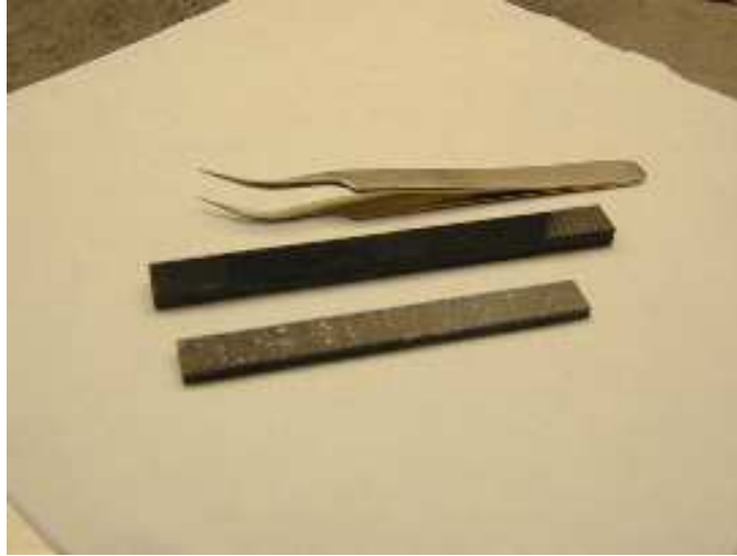
Figure 6.6: Sintered silicon carbide before (up) and after (down) annealing at 1900 C. The upper is cantilever 4, the lower cantilever 3.
