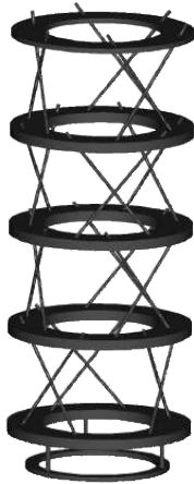
Figure 3.4: Lattice structure. The TF lattice structure is formed by four stages with cylindrical symmetry. Each stage holds a thermal radiation shield, not shown in the picture.
