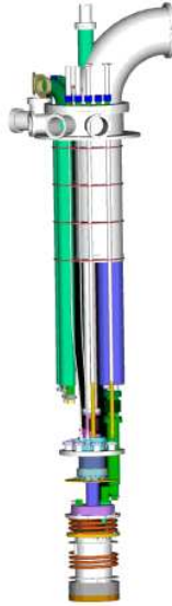
Figure 3.9: A view of the TF dilution refrigerator. It spreads through all the TF length: it passes through the honeycomb, the Dewar and the IVC flanges, the radiation shields and the cryogenic suspensions.
