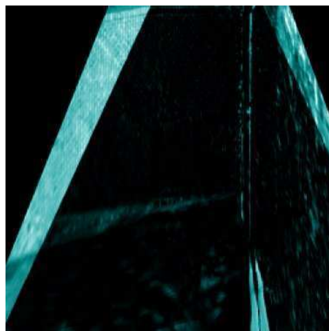
(e) Resulting disparity map. The building edge appears clearly at the bottom of the image.
