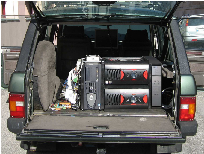
(a) Visible, from left to right: the safety device (orange), the power electronics board (mounted upright), the control PC, the two stacked vision PCs, and the UPS power supply.
