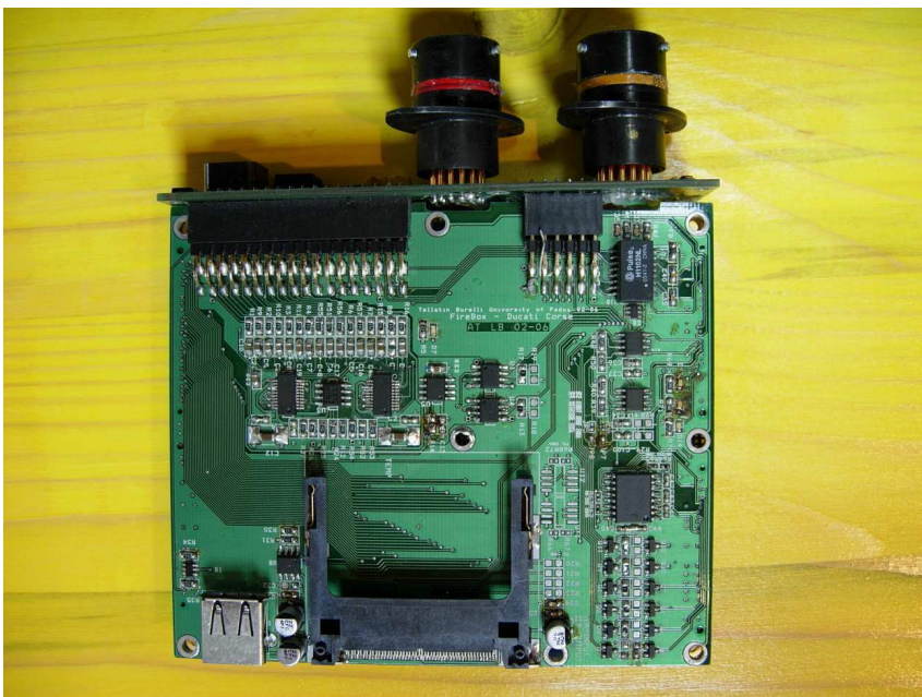
Figure 7.4: The analog electronics and CompactFlash slot on the host board. The black mating elements with the connector board are visible on top.
