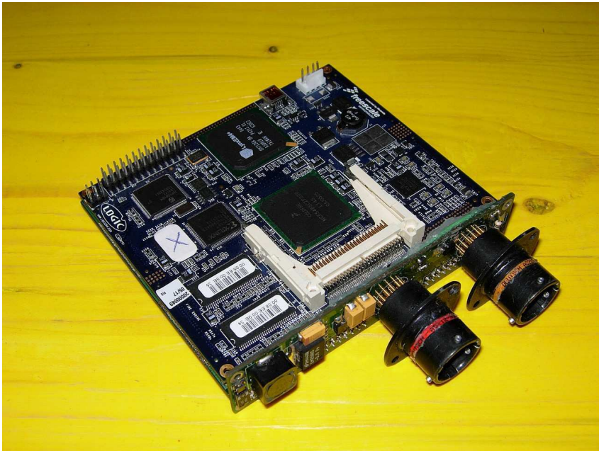
Figure 7.3: The assembled device, showing the Fire Engine CPU board and the board with the Deutsch connectors and the power supply.
