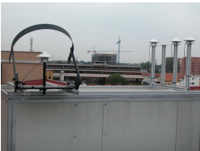
Figure 4. Pyranometers for global and diffuse solar radiation.
