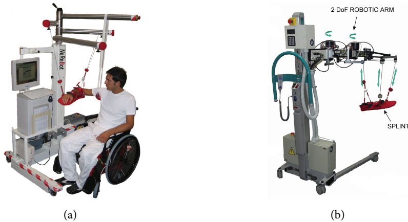
Figure 1.11: The 3D wire-based rehabilitation devices designed at DIMEG: NeReBot [66, 51] (a) and MariBot [22, 67] (b).
