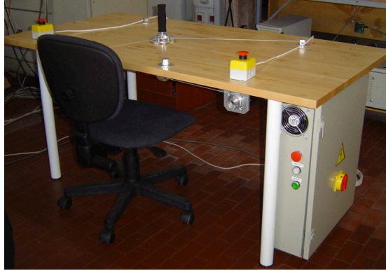
Figure 1.12: The first planar cable-based rehabilitation device developed at DIMEG: Sophia-4 [72, 73].
