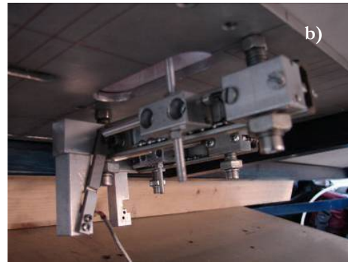
Fig. 6.13 – a) On the left, the protected load cell installed on the support under the upper plane that measured the impact force against the rear structure; b) on the right, the non-protected load cell that measured the impact force against the front structure.
