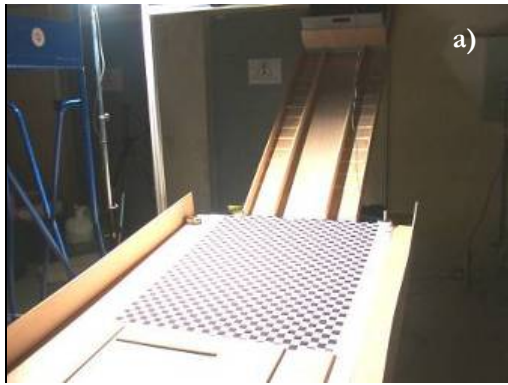
Fig. 5.42 – a) On the left, view of the white and black chess paper panel; b) on the right, Reference image – Calibration in the plane (x,y) , white and black chess paper panel image.
