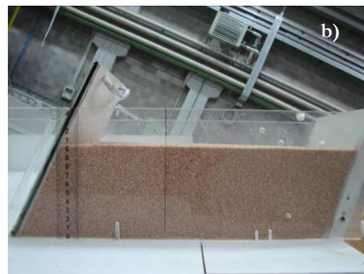
Fig. 6.9 – a) On the left, the feeding box with 3 kg of granular material; b) on the right, the feeding box with 7 kg of granular material.
