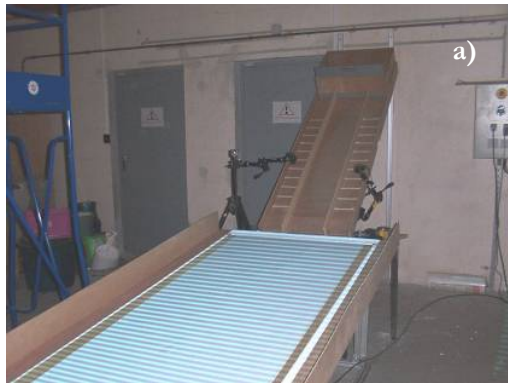
Fig. 5.43 – a) On the left, view of the lower plane with the fringes projected; b), c), d), e) below, four images taken with the video camera (video camera III), Reference images – Calibration along z , lower plane images ( z = 0 ) with the phase shift of 0, \pi/2, \pi, 3\pi/2 .
