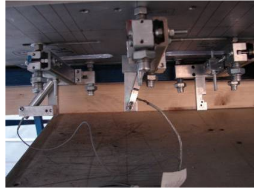
Fig. 6.36 – Two views of the support plate with the three T-shaped supports below the upper plane.
