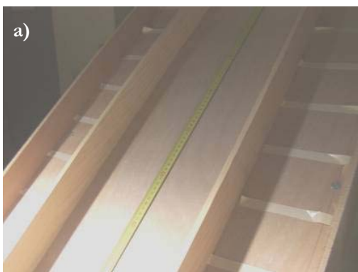
Fig. 5.34 – a) On the left, view of the channel with the ruler positioned in the centre of the channel; b) on the right, Reference image – Calibration in the plane (x, y) , ruler image.
