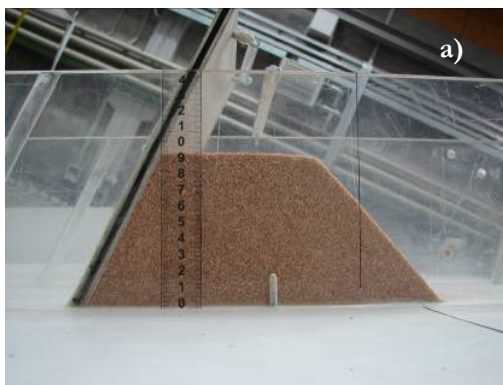
Fig. 6.9 – a) On the left, the feeding box with 3 kg of granular material; b) on the right, the feeding box with 7 kg of granular material.
