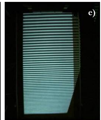
Fig. 5.43 – a) On the left, view of the lower plane with the fringes projected; b), c), d), e) below, four images taken with the video camera (video camera III), Reference images – Calibration along z , lower plane images ( z = 0 ) with the phase shift of 0, \pi/2, \pi, 3\pi/2 .
