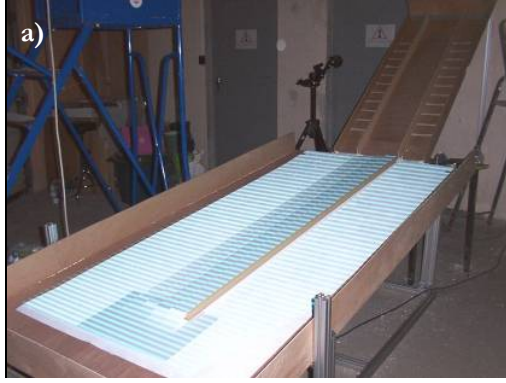
Fig. 5.44 – a) On the left, view of the lower plane with the fringes projected and the boards of wood positioned in the centre of the plane; b), c), d), e) below, four images taken with the video camera (video camera III), Object images – Calibration along z , four images of the boards ( z = 0,9 ; 1,9 ; 3,0 ; 4,0 ) with the phase shift of 0, \pi/2, \pi, 3\pi/2 .
