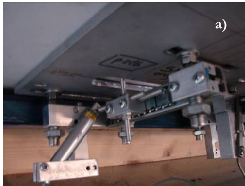
Fig. 6.13 – a) On the left, the protected load cell installed on the support under the upper plane that measured the impact force against the rear structure; b) on the right, the non-protected load cell that measured the impact force against the front structure.
