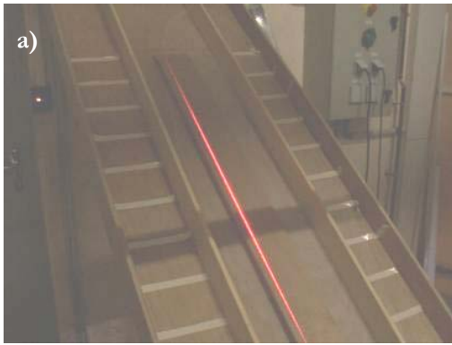
Fig. 5.35 – a) On the left, view of the channel with the laser line in the centre of the channel; b) on the right, Reference image – Calibration along z , channel plane image ( z = 0 cm).
