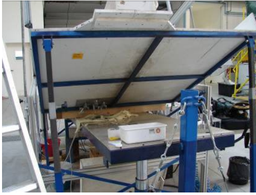
Fig. 6.36 – Two views of the support plate with the three T-shaped supports below the upper plane.
