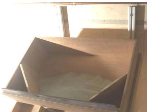
Fig. 5.11 – Two views of the feeding box with 10 kg of granular material.
