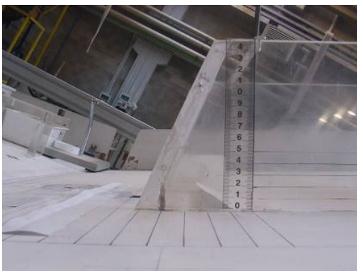
Fig. 6.18 – The measuring section of the tests. The measuring section is fixed at 108 cm from the feeding box (section 0 cm).
