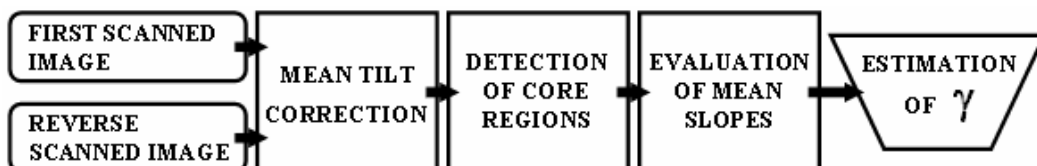
Figure 4.15: Orthogonality estimation procedure.
