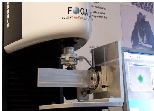
Figure B.6: A picture of the rotational stage, integrated with the optical profilometer.
