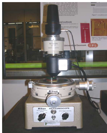
Figure B.3: A picture of the open loop AFM mounted on a conventional stage.
