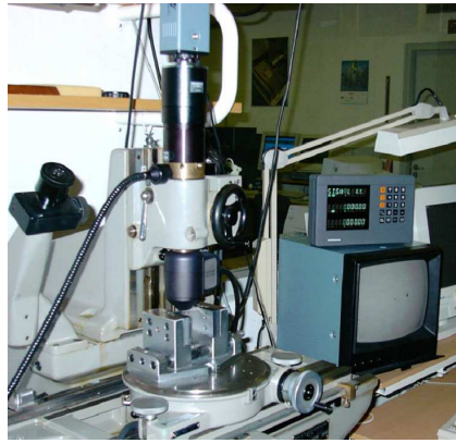
Figure B.2: A picture of the Large range AFM during operation. The AFM is mounted on the z axis of the CMM. On top of the scanner, a CCD camera is used for positioning. The readout of the electronic scales can be discerned on the right side.
