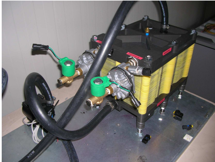
Figure 5.1. Detail of the fuel cell stack before installing it. The gas inlets with their pressure regulators and the solenoid valves are on the left of the stack. The electrical terminals are located on the top (negative) and on the bottom (positive) of the stack. The black pipes carry the coolant (demineralised water).
