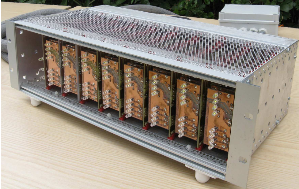
Figure 5.19. Picture of one of the racks for the acquisition of up to 64 fuel cell element voltages. From left to right: the first board is the microcontroller board, the other eight ones are the multiplexer boards. The LEDs on the front display the power supplies and the signal selection.
