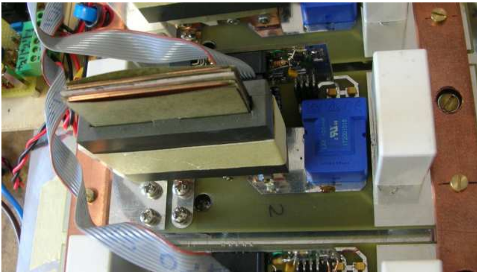
Figure 5.6. A detail of one of the six modules. The MOSFET and the diode are located under the main board, in contact with the aluminium heat sink.
