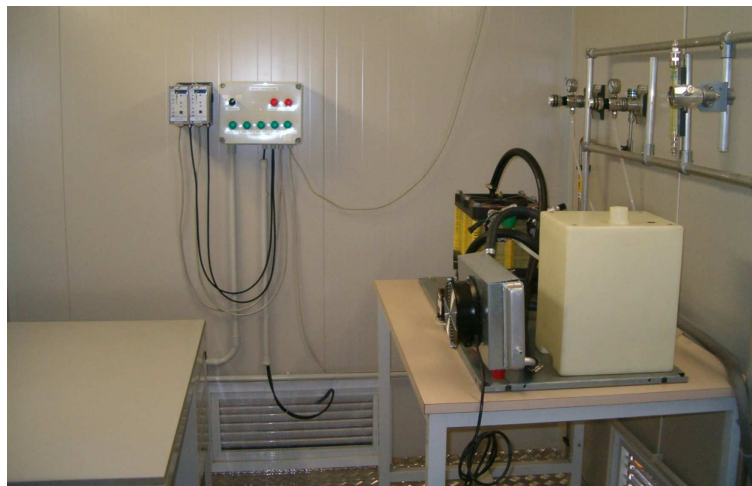
Figure J.3. The table on the right is for the fuel cell stack under test. The table on the left is for the power electronics converter connected to the fuel cell stack.
