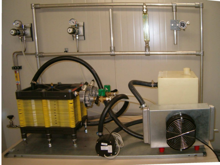
Figure J.9. Fuel cell stack and fittings before installation.
