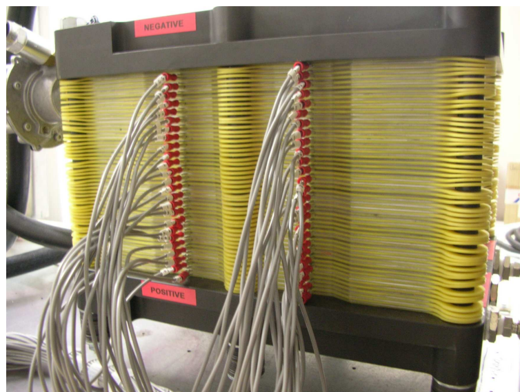
Figure 5.3. A detail of the fuel cell stack, showing 51 wires used to acquire and measure the 50 differential voltages of every single element.
