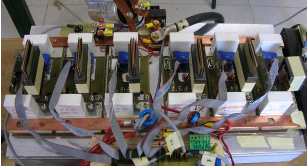
Figure 5.5. The boost prototype with its input bars on the rear side and its output bars on the front side. The six modules are visible, each with its input and output capacitors, its inductance, its current sensor and its current control board.
