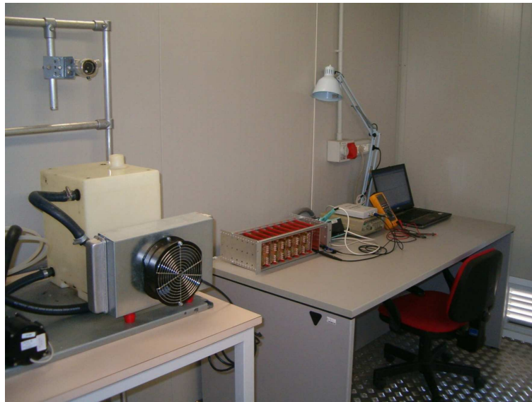
Figure J.2. The table on the right is for the computerised controller system. The table on the left is for the fuel cell stack being tested.
