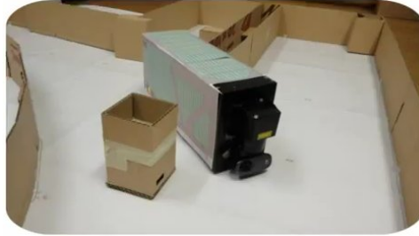
Figure 4.2: ITER model vehicle prototype equipped with laser and camera.
