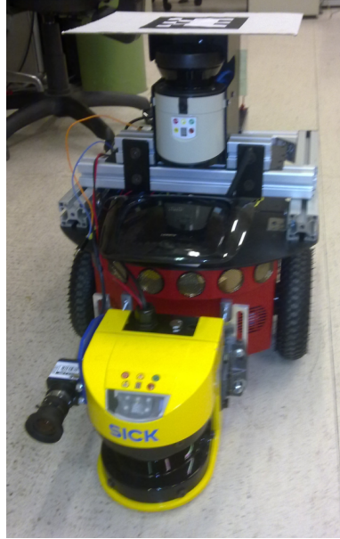
Figure 4.1: Mobile Robots Pioneer P3-DX test vehicle equipped with lasers and camera.
