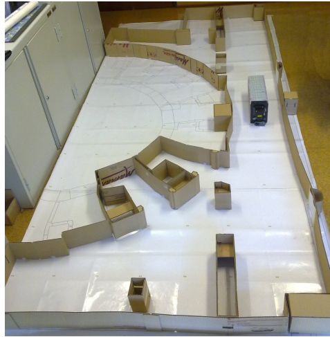
Figure 4.12: Environment and CPRHS mobile robot mock-up used to collect data for the experimental results.
