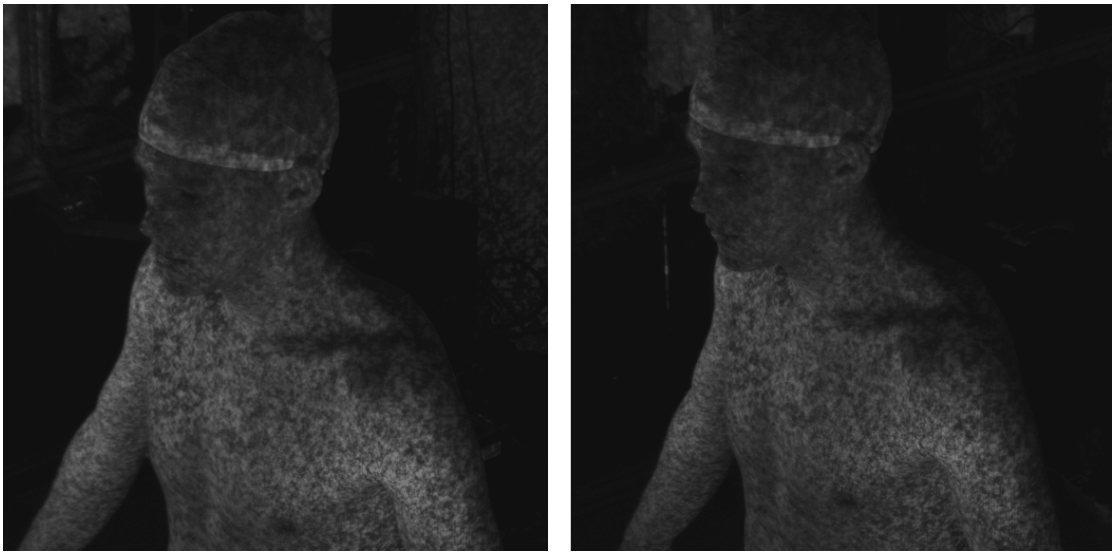
Figure 6: Example of projected speckle pattern captured by a pair of stereo cameras.
