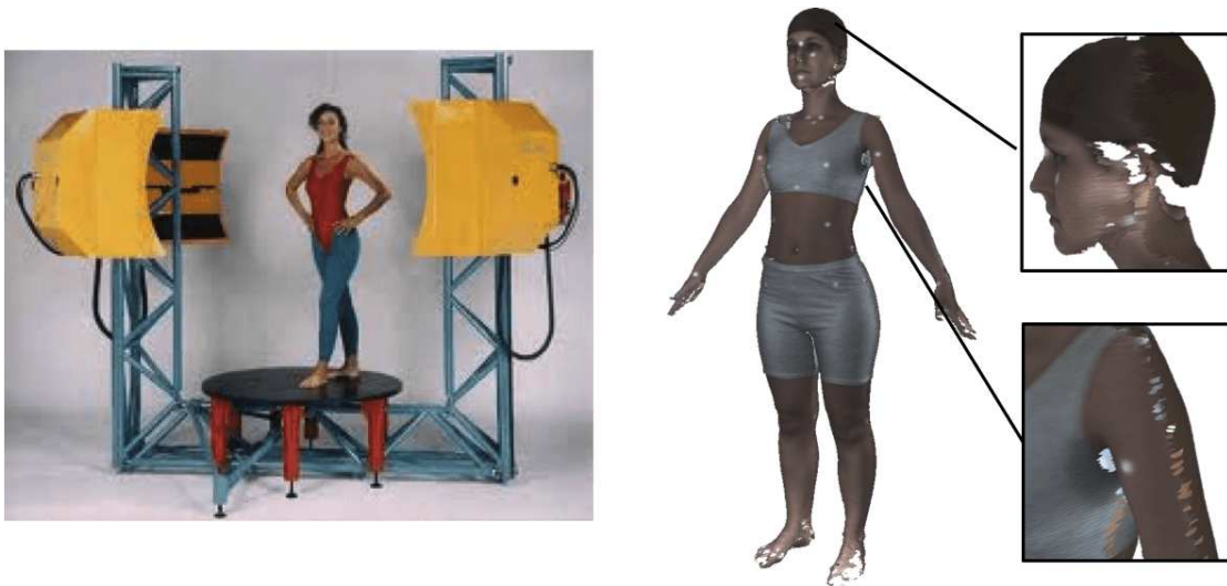
Figure 4: A full-body laser scanner from Cyberware [3] and a laser scan from the CAESAR dataset [107] (scan resolution: 124825 vertices). 3D reconstruction may be imperfect in areas that are either unreachable by the laser or invisible by the camera.
