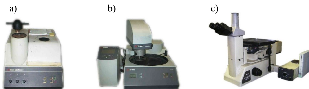
Figure 2.6. Images of metallographic analysis apparatus. Metallographic compression mounting press (a), automated polishing machine (b), inverted reflected light microscope interfaced with image analysis software (c)
