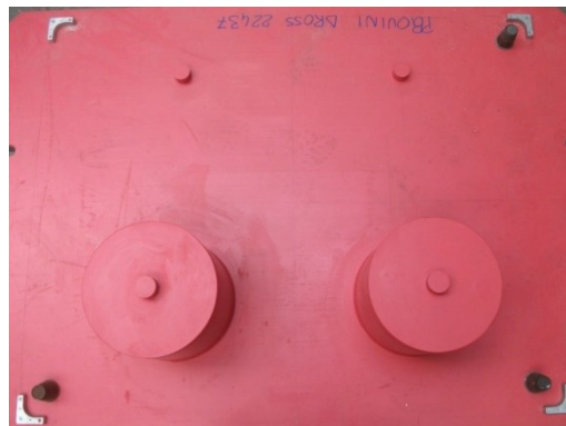
Figure 2.2. Geometry of the pattern of the cylinder \varnothing 300 mm, h 520 mm.
