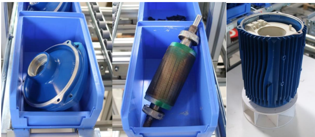
Figure 37: Parts of the horizontal multistage centrifugal electric pump. From the left: seal housing disc, pump rotor, pump crankcase
