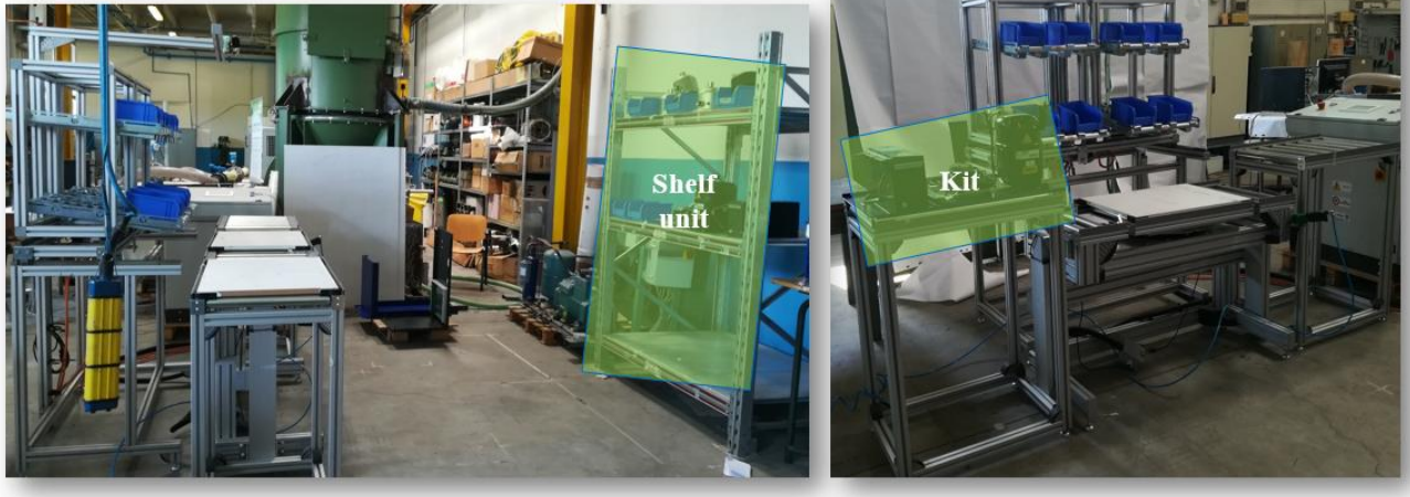
Figure 31: Assembly system configuration with line stocking (left) and kitting (right)
