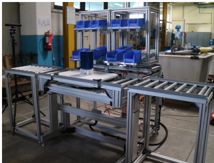
Figure 34: SASAS equipped with Microsoft Kinect™
