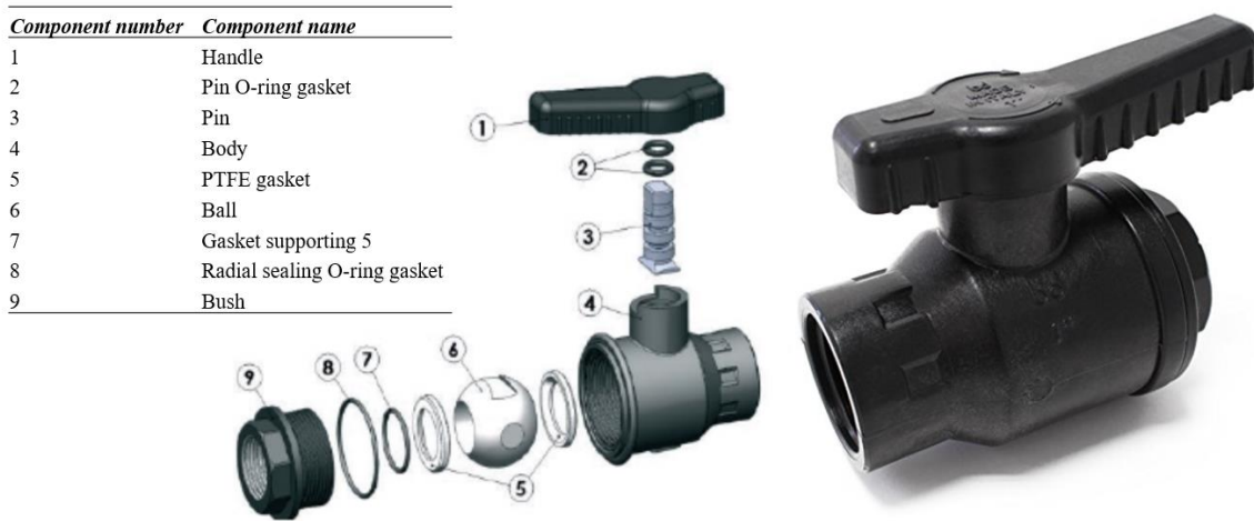
Figure 8: Example of a valve variant and its components
