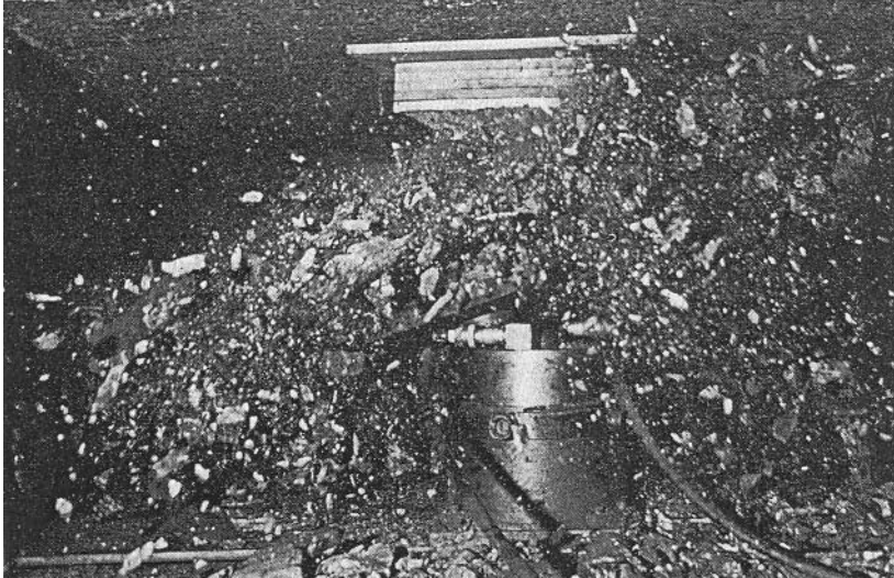
Figure 2.5. Explosion of a coal specimen during an on-site unconfined compressive test, from Bieniawski (1968).
