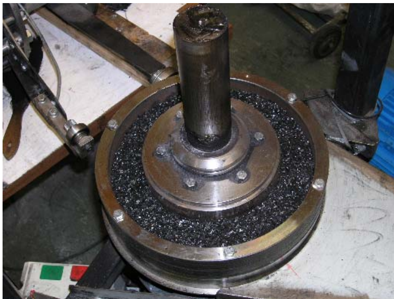
Figure A.5 A sample of coal granules loaded in the rheometer's bowl
