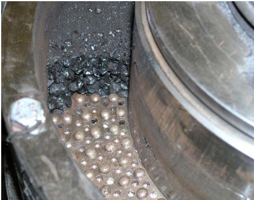
Figure 3.4 Situation of the sample (in this case coal granules) after a test: a layer of unfragmented material remains in contact with the bowl floor, while a thin layer of coal dust coats the sample.
