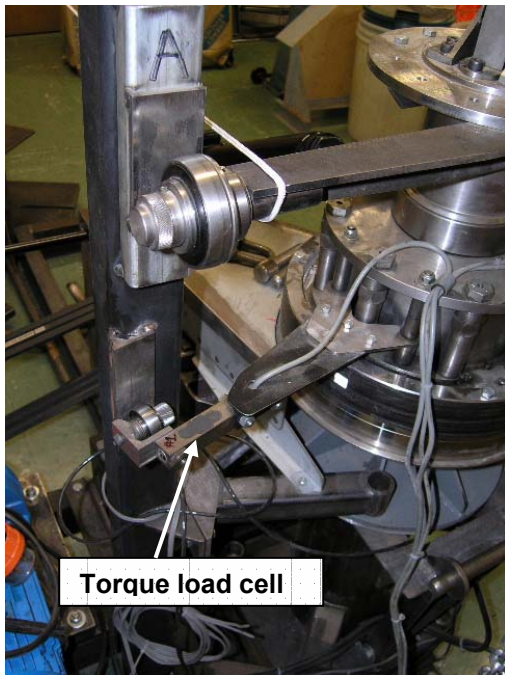
Figure A.3 Calibration of the torque load cells, particular.
