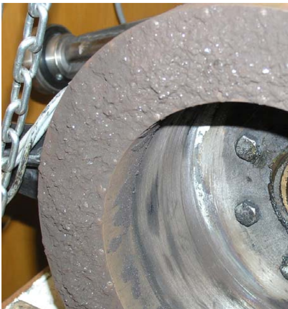
Figure 3.12 Compacted coal dust on the inner side of the cover plate after a test
