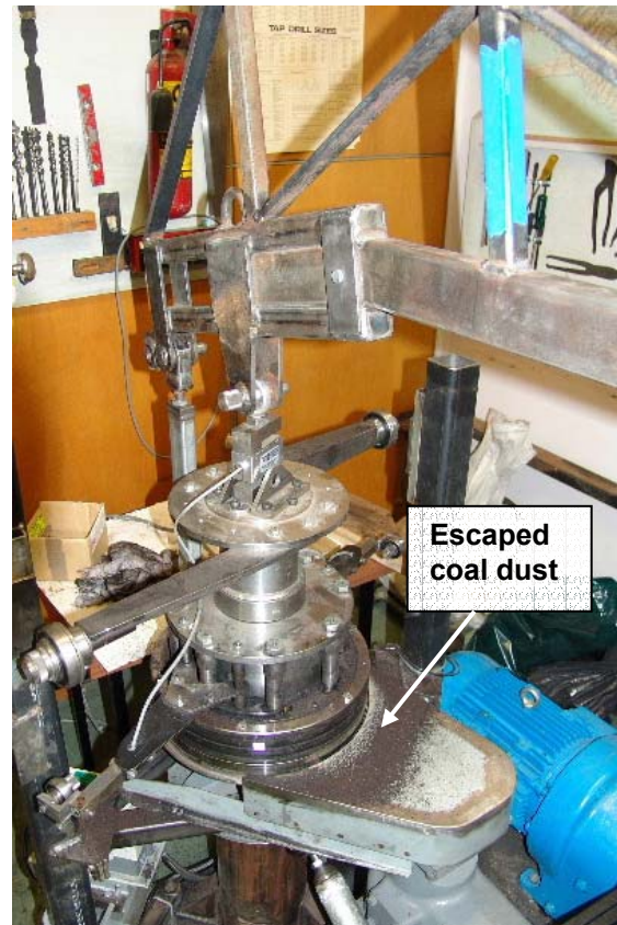
Figure A.4 The rheometer after a test with coal grains.
