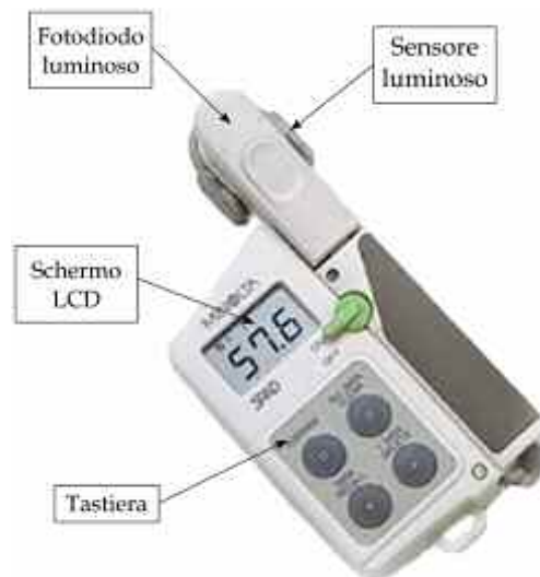
Figura 9 - Minolta Chlorophyll Meter SPAD-502.
