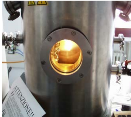
Figure 3.7. Electron Beam Deposition Facility at LUXOR
