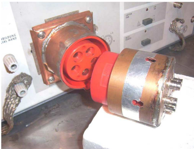
Figure 4.8: Type B proposed adapter for the calibration of LISN input impedance.
