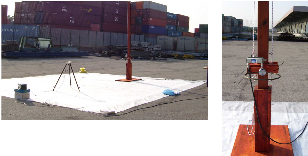
Figure 3.17: The OATS realized at the C.R.E.I. Ven facility and the sliding support on the mast
