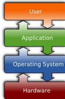
Figure 1.1: A layer structure showing where Operating System is located on generally used software systems on desktops
